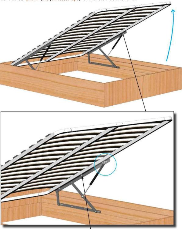
6. Use the slots on the lift mechanism to adjust the position of the frame.
